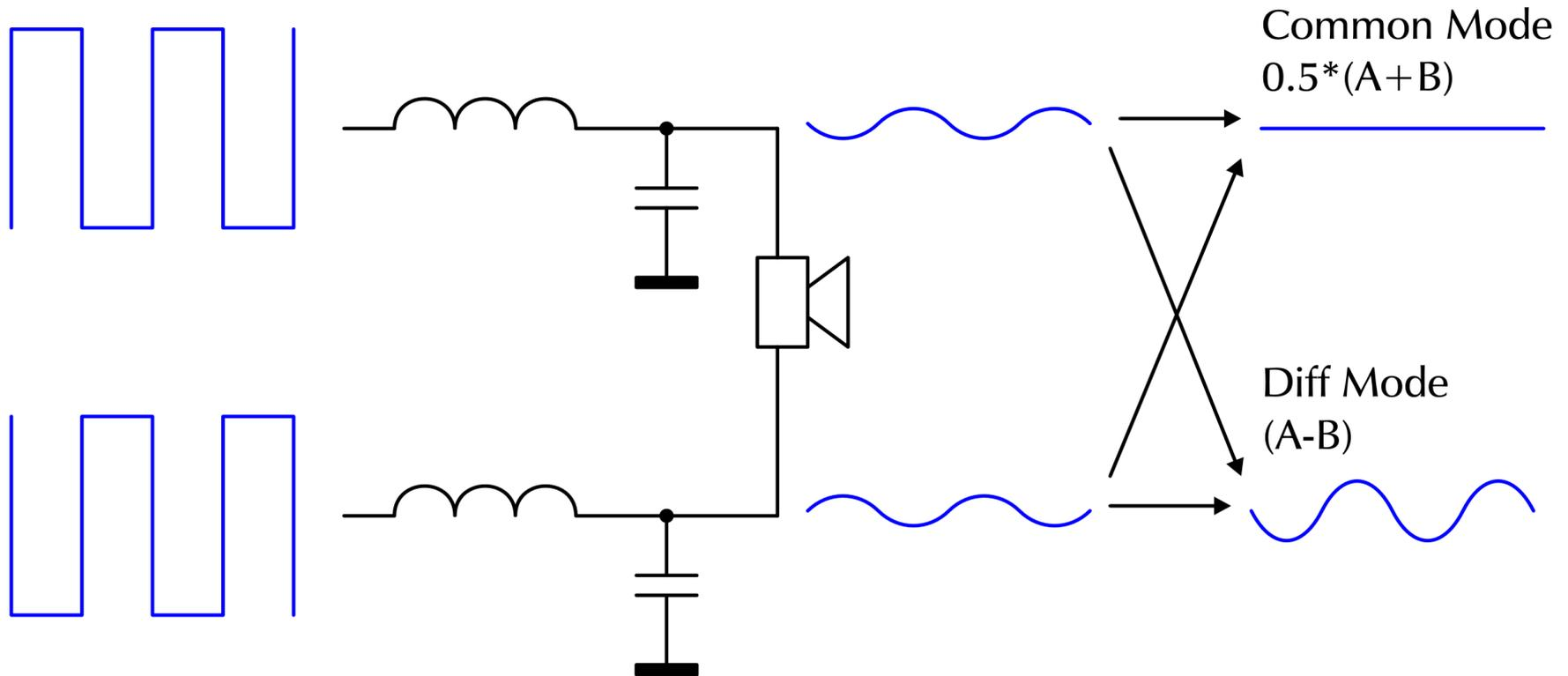
Note: Common-mode is what radiates off cables.
