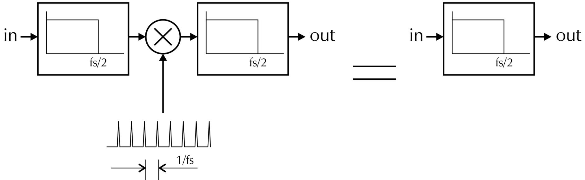
*A sampler flanked by low-pass filters with sufficient attenuation at  $f_s/2$  does exactly the same as the low-pass filters alone.*
