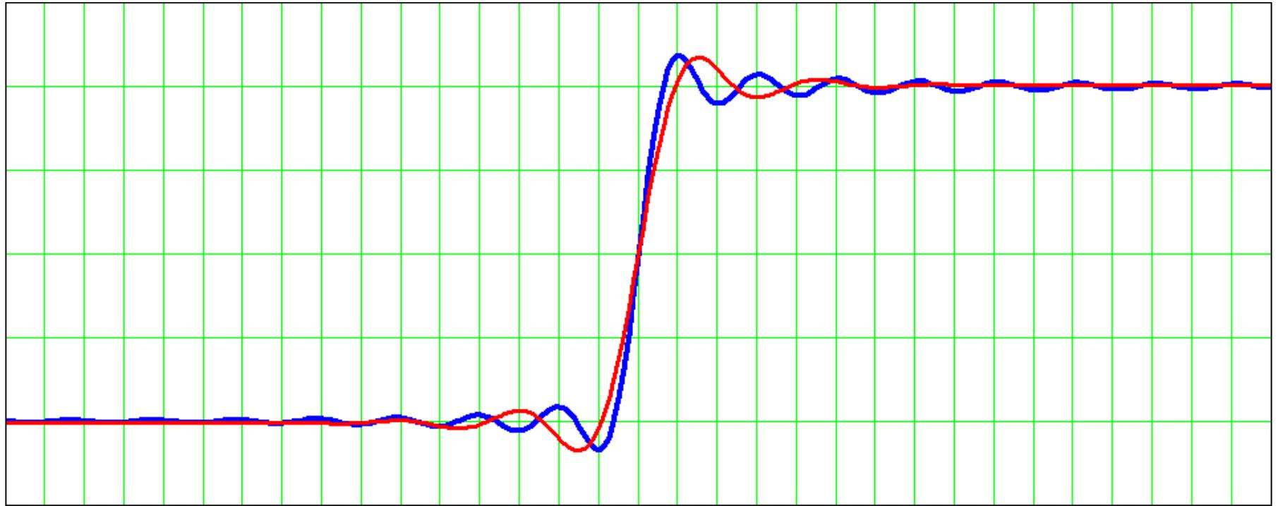
(example: standard 96kHz AD/DA with slow LPF inserted)
